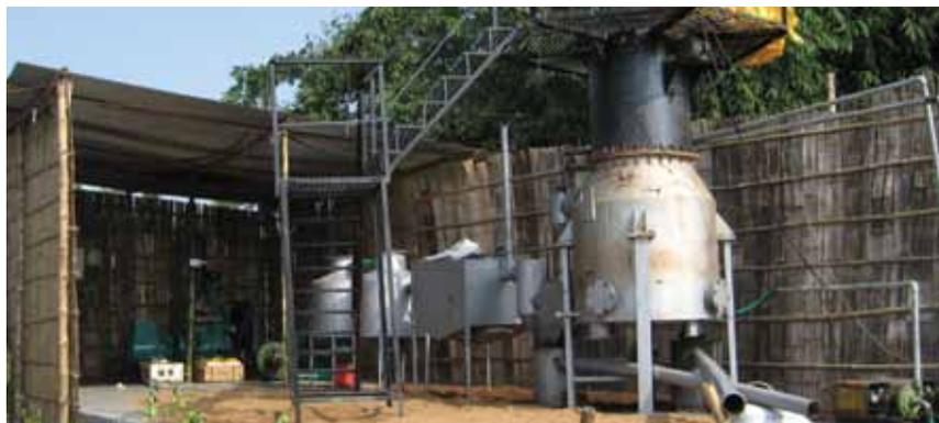
Husk Power Systems has pioneered a new way of providing electricity to rural India through the gasification of rice husk.
